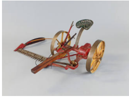
Title: Model of Horse Drawn Mower Medium: Painted and enameled brass, steel, iron
