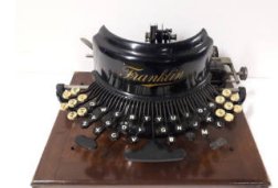
Title: Typewriter Primary Maker: Franklin Typewriter Company Medium: Steel, nickel, leather, rubber, celluloid, oak, tin
